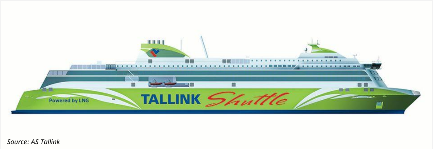
Tallink's new LNG-fuelled, high-speed, shuttle ro-pac ferry will serve the Tallinn-Helsinki route from 2017, with a 17 knot service speed
