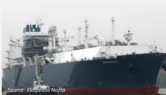
Lithuania's New 170,000 m 3 LNG FSRU, "Independence"
