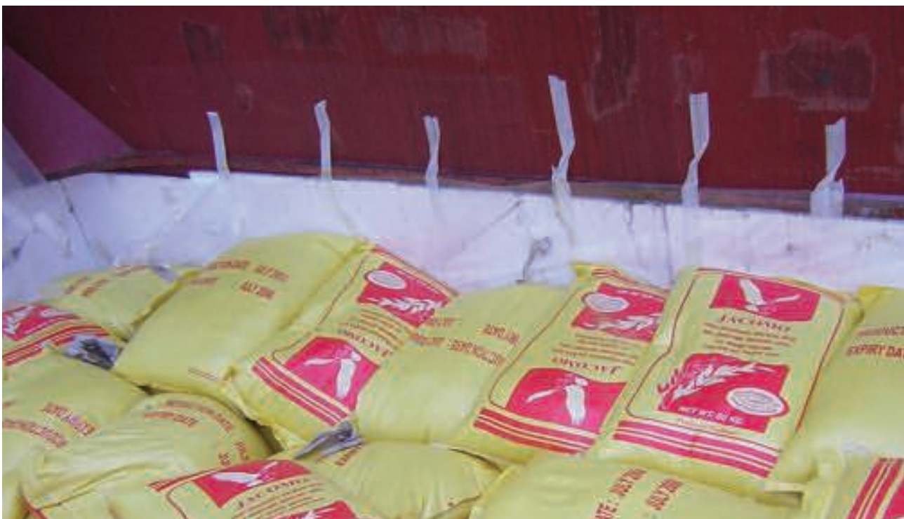
Styrofoam boards and plastic sheeting used in the Allied Maritime dunnaging arrangement
