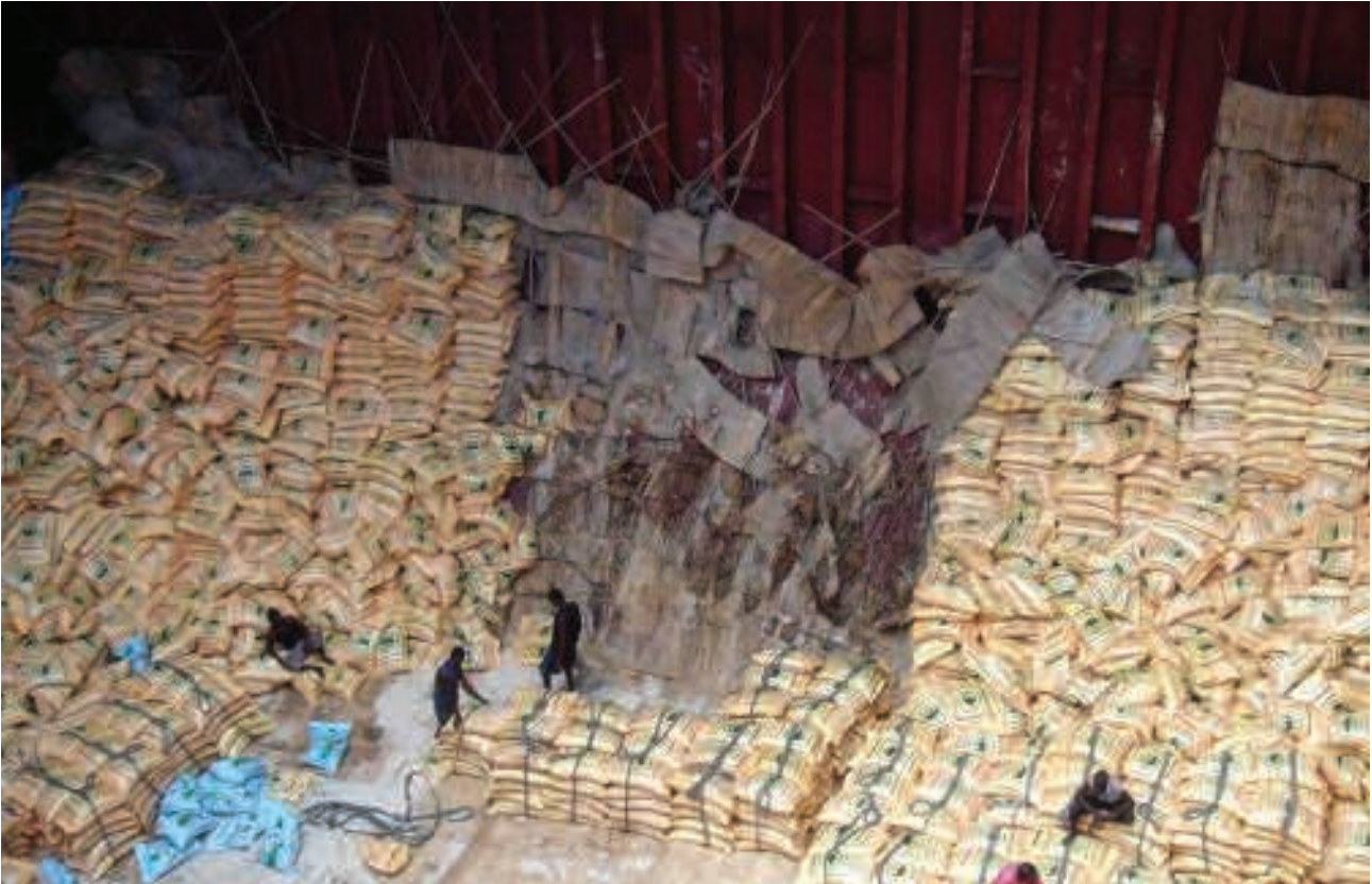
Traditional dunnaging arrangement with evidence of the passage of moisture over the lower hopper
