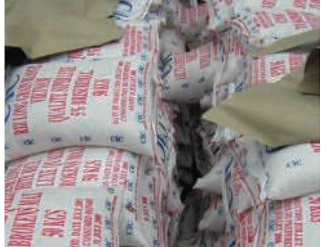
Typical athwartships ventilation channel. However, experts question whether ventilation channels are necessary at all
