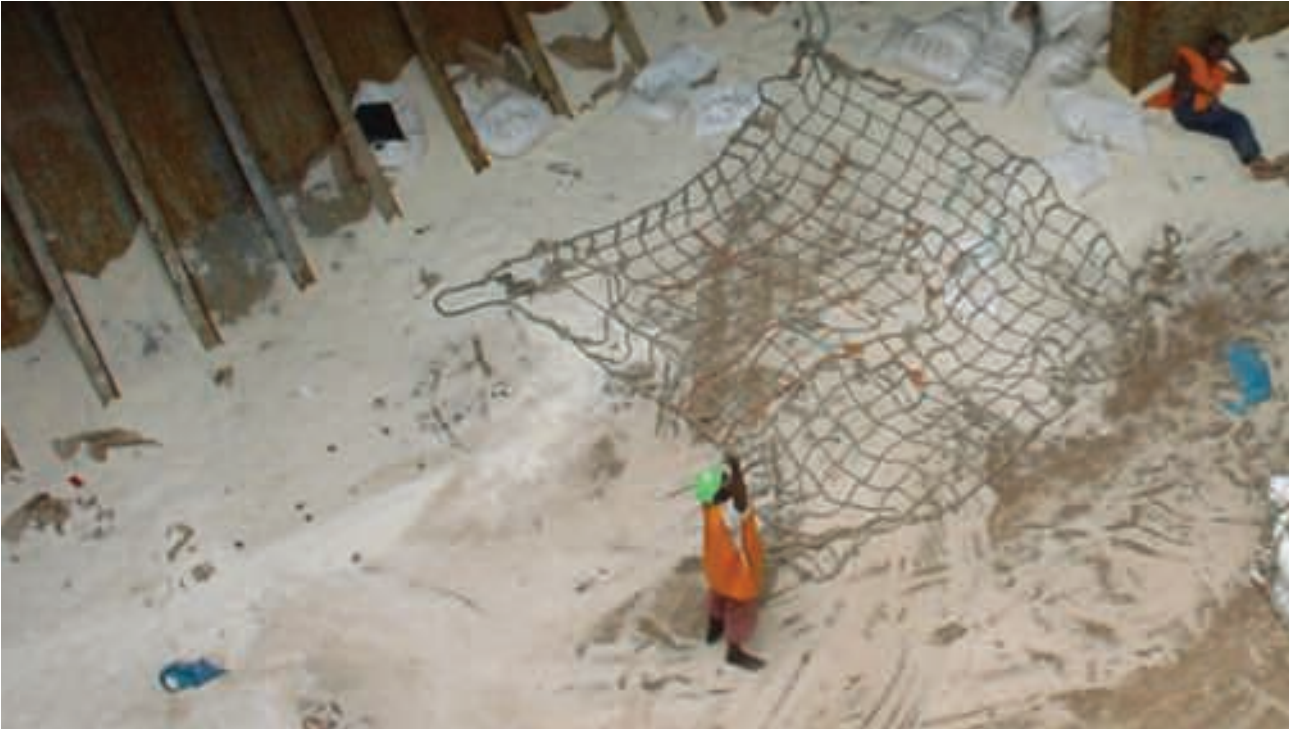
Large quantities of sweepings may give rise to an apparent shortage due to overfilling of bags
